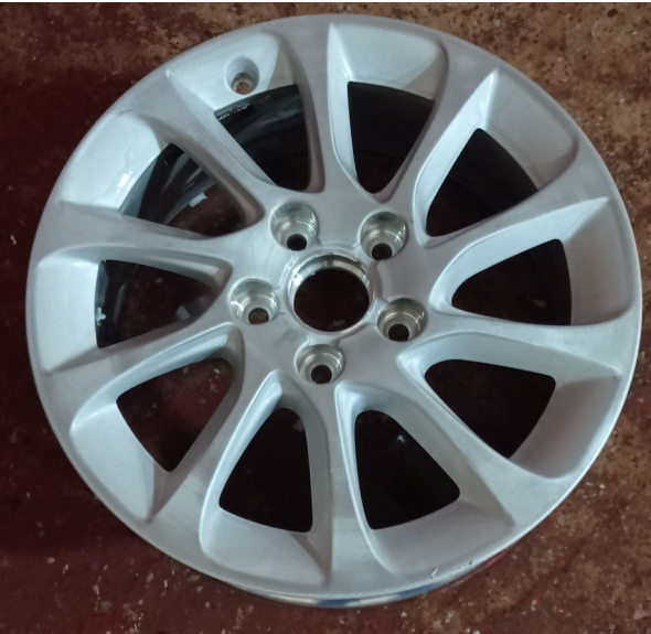
Figure 6: 6 Hours at 65 °C – Paint has fully stripped despite lower tank temperature
