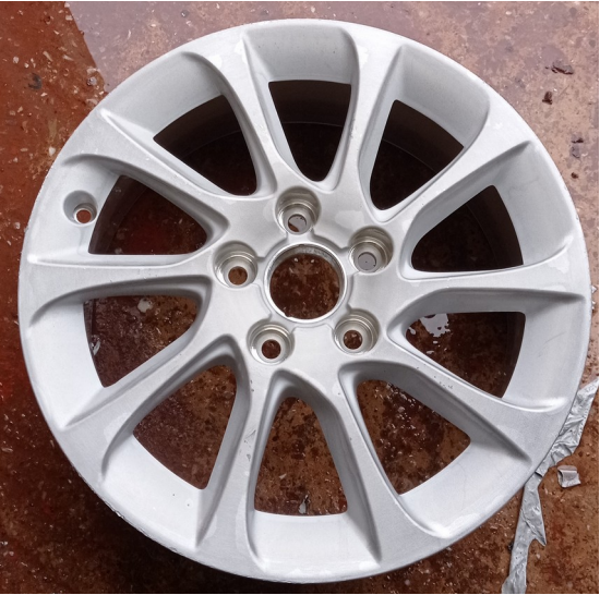
Figure 3: 4 Hours at 72 °C – After jet washing the paint has been fully removed with a finish comparable to Fig.2
