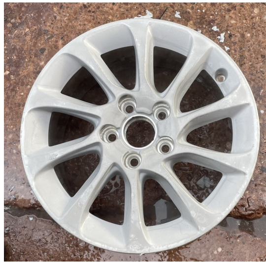
Figure 2: 2 Hours at 80 °C – After jet washing the paint has been fully removed
