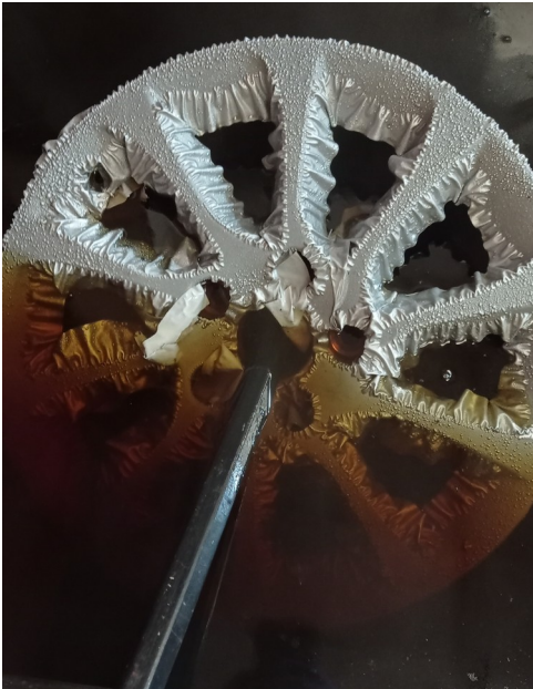
Figure 5: 4 Hours at 65 °C – Paint is beginning to lift from the wheel
