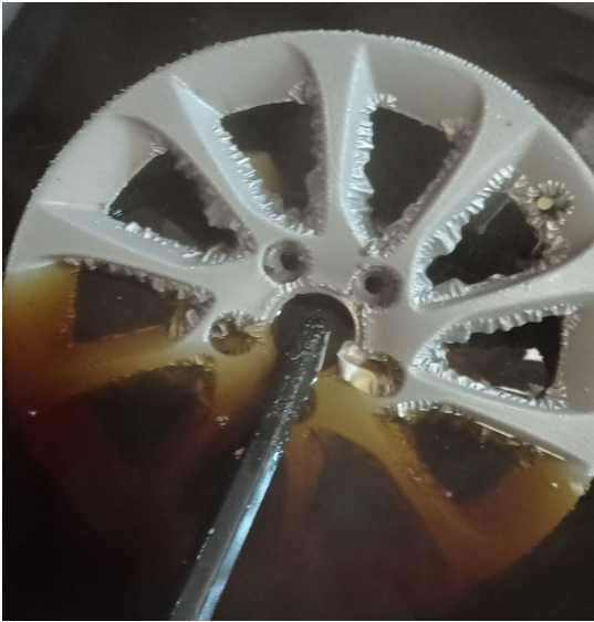
Figure 4: 2 Hours at 72 °C – Slight lifting of the paint can be observed. At the half way mark less paint has lifted when compared to Fig.1
